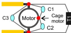
Power Under-voltage. Solder Low ESR 470-2200uF capacitor to the power input leads of the ESC.
